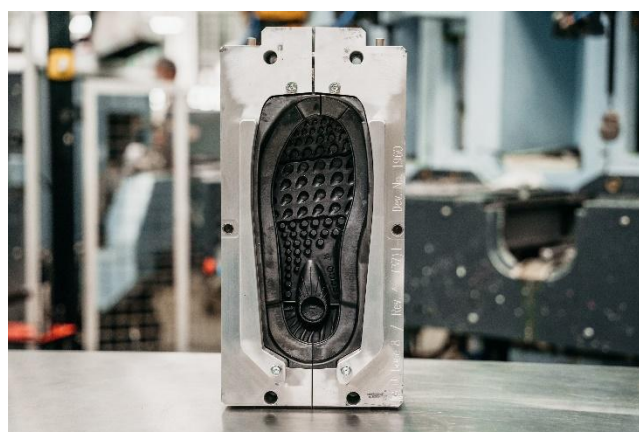
Figure 3: ECCO accelerates product development by including Stratasys Origin One 3D printers (3D print outsole). Source: Businesswire, 2021.
