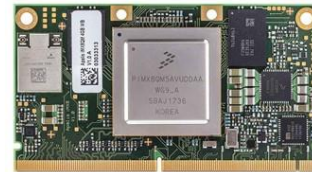
NXP i.MX8QM with a GPU + 6x Cortex-A CPU cores
