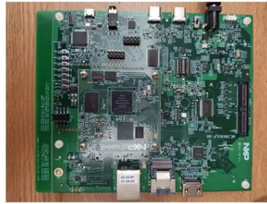
NXP i.MX8ULP (ultra-low power microprocessor with a DSP)
